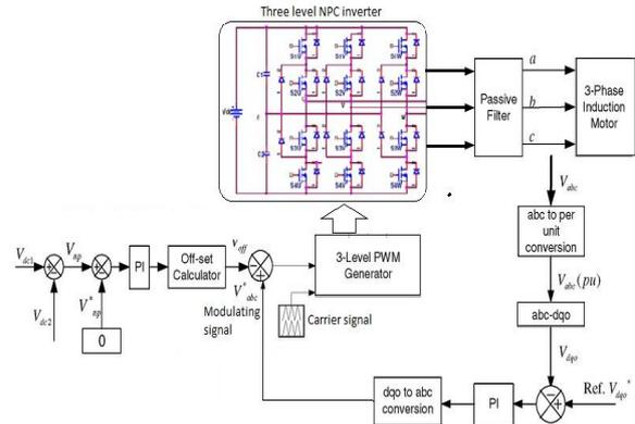
Fig.3 NPC offset addition PWM block diagram
