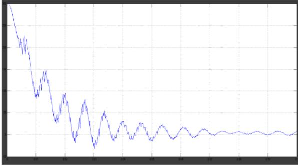
Fig.11 Neutral point voltage ( $V_{np} = V_{dc1} - V_{dc2}$ )
