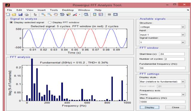
Fig.9 Simulated inverter line voltage (Vab) and its frequency spectrum with unbalanced dc link with neutral point balancing after filtering.
