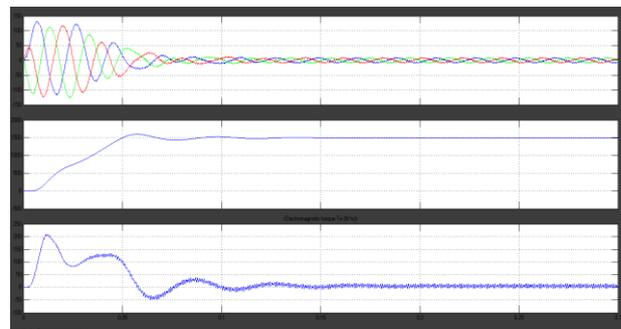
Fig.10 Stator current waveform (Ia, Ib and Ic) , Motor speed (rpm), Electromagnetic torque waveforms under balanced dc link voltages after neutral point voltage balancing.
