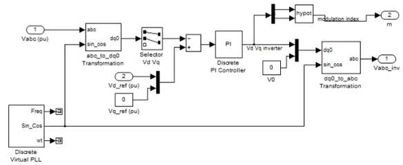
Fig.4 abc to dqo conversion reference comparison and dqo to abc conversion
