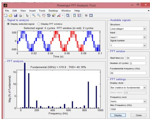
Fig.7 Simulated inverter line voltage (Vab) and its frequency spectrum with unbalanced dc link without closed loop offset PWM and
