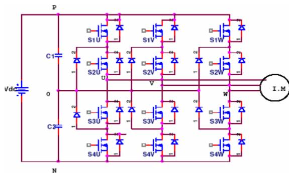
Fig.1. Three phase three-level NPC.
