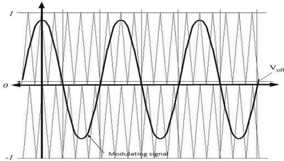
Fig.5 Offset addition PWM
