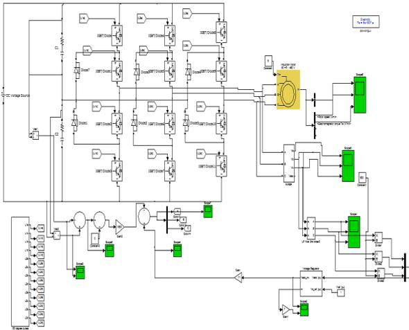
Fig.6 A MATLAB/Simulink model of three-phase three-level DCMLI with the carrier-based offset addition PWM
