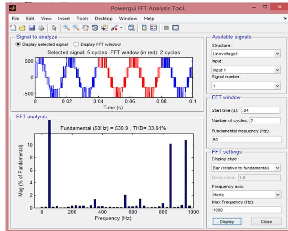
Fig.8 Simulated inverter line voltage (Vab) and its frequency spectrum with unbalanced dc link with Neutral point balancing.
